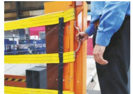
**3** When Vehicle Restraint System securely connects the vehicle, the inside traffic light turns green, the dock safety barrier interlock releases, allowing for loading and unloading of a trailer.
