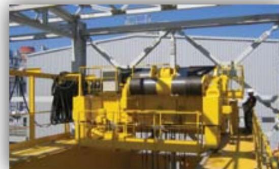
❖ **Crane Modifications and Conversions:** Where existing cranes are to be re-used in another location or due to change in the crane application, we can provide the consultation, design and execution of crane modifications. These include increased lifting capacities, changes in structural dimensions, modernisation of control systems, conversion to radio remote control and replacement of obsolete components. The works can be done at clients site or in our factory.
