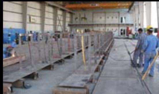
❖ **Crane Manufacture and Assembly:** In-house girder fabrication, shotblasting, painting and crane assembly. Welding procedures, non-destructive testing including radiography and crane functional testing. Our facility is approved by major companies such as Dubai Aluminium, General Electric, Alstom. Our Quality Management System is certified to ISO 9001-2008.
